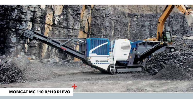
The MC 110 R EVO's advantages include considerably high power in its class and its vibrating feeder with integrated slotted grate. The plant is used as a primary crusher for natural stone as well as in demolition and recycling companies. Thanks to its low weight, it is easy to transport and flexible in operation.
