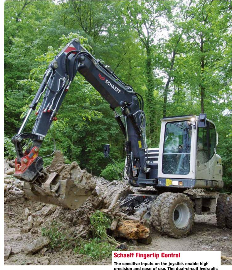
precision and ease of use. The dual-circuit hydraulic system with load independent flow sharing (LUDV) allows simultaneous, independent work movements. Economic load sensing technology ensures accurate volume control, hence saving fuel.
